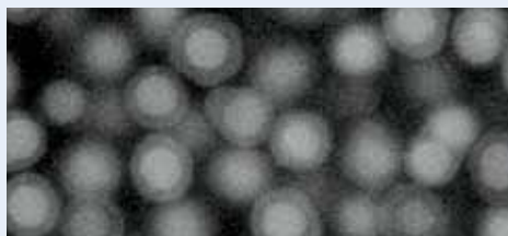
FIGURE 5: Scanning electron microscope (SEM) photograph of HALO particles
