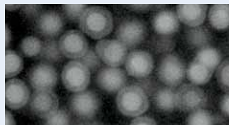
FIGURE 7: Scanning electron microscope (SEM) photograph of HALO particles
