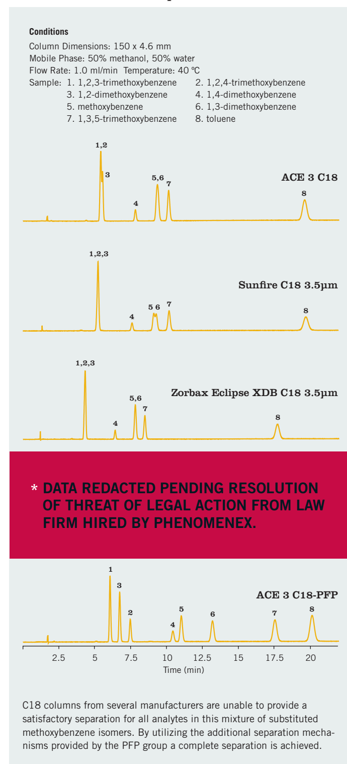
FIGURE 10: Achieving a better separation by applying additional mechanisms of separation
