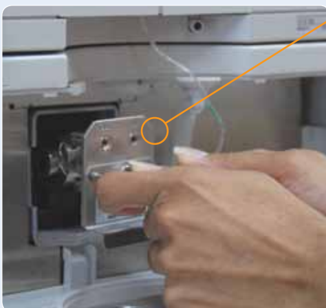
FIGURE 5: Replace standard detector flow cell with either a semi-micro flow cell (low ECV configuration) or a micro flow cell (ultra-low ECV configuration).
