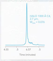
Improved resolution of an IgG1 (trastuzumab) is demonstrated by the 2.7  $\mu m$  particle with 1000 Å pores. This is not unique to this antibody.
