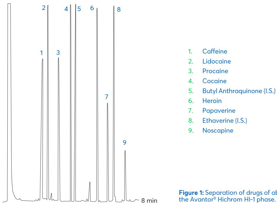
**Figure 1:** Separation of drugs of abuse using the Avantor® Hichrom HI-1 phase.
