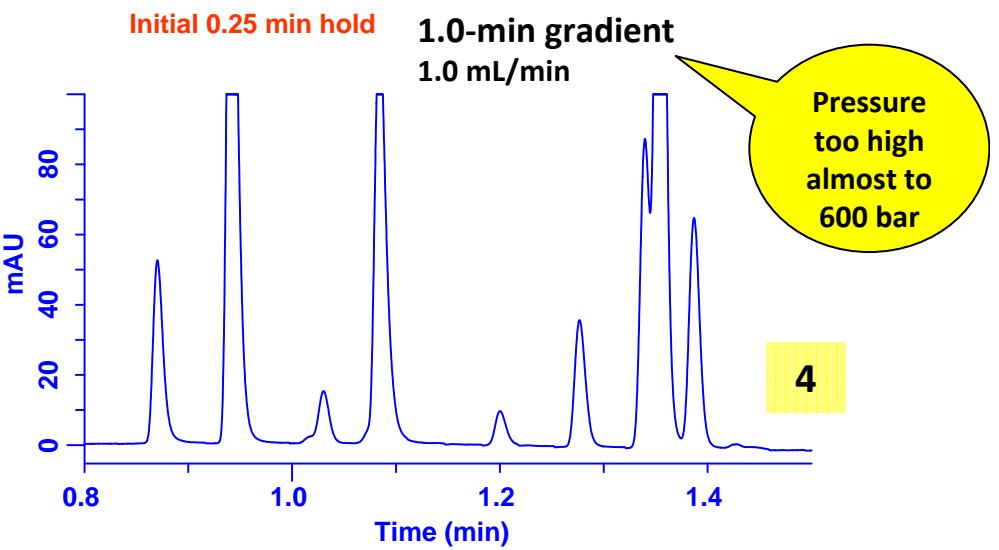
15–80% MeOH/0.1% HCOOH, 10 mM NH<sub>4</sub>COO, 40°C, 1 µL inj., 2 µL flow cell, 80 Hz
