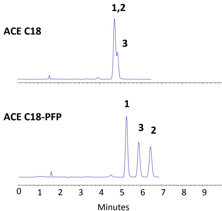
ACE C18-PFP shows additional separation mechanism compared to C18 columns
