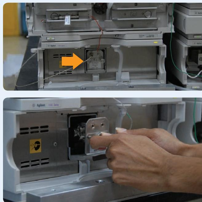
Replacing the detector flow cell in an Agilent 1100 is simple. It is readily accessible and has just two thumb screws holding it in place.
