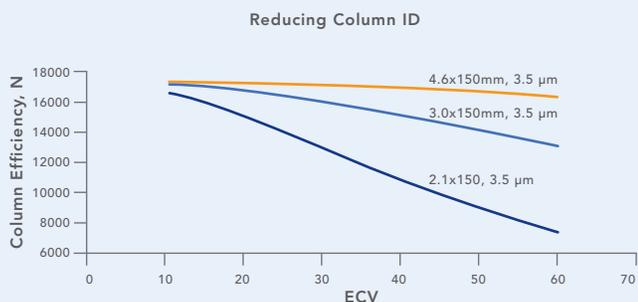
Reducing column ID is a great way to reduce solvent consumption, but the smaller the column ID the more susceptible the column is to ECV. All three of these columns have approximately the same efficiency, but the 2.1 mm ID column could have an “observed” efficiency over 30% less than that of the 4.6 mm ID column when used with typical conventional HPLC equipment with ECV greater than 30  $\mu\text{L}$ .
