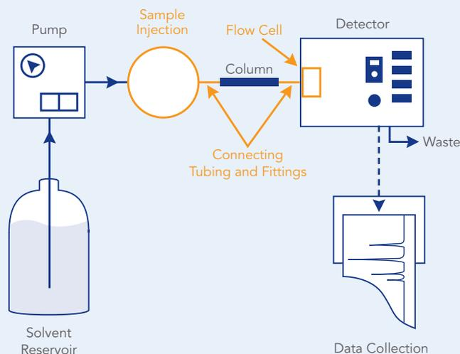
In this schematic of an HPLC system, the gold color indicates where extra column volume, ECV, is located.
