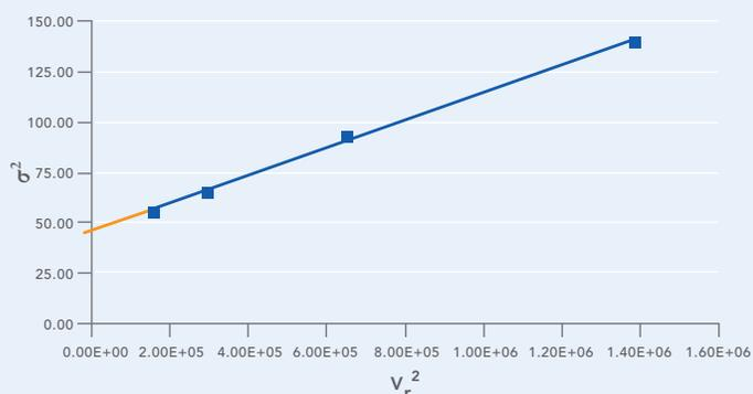
Y-intercept =  $\sigma_{ec}^2 = 43$       ECV =  $4 \times \sigma_{ec} = 4 \times 6.6 \mu\text{L} = 26 \mu\text{L}$
