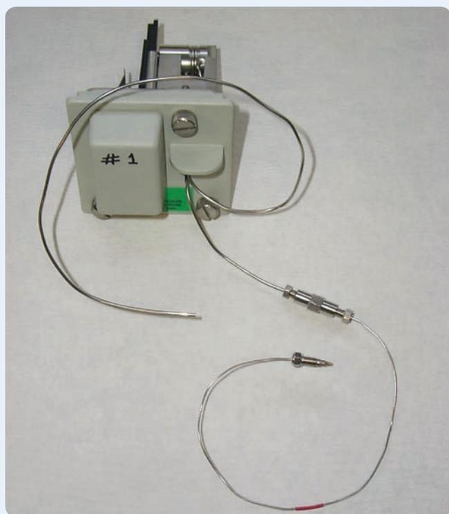
The Waters Alliance 2487 detector is shown sitting on top of the Waters Alliance system in the top photo. Removing the cover of the detector allows access to the detector flow cell assembly, shown in the bottom photo. Two screws hold the flow cell assembly in place, making it easy to install a smaller volume flow cell.
