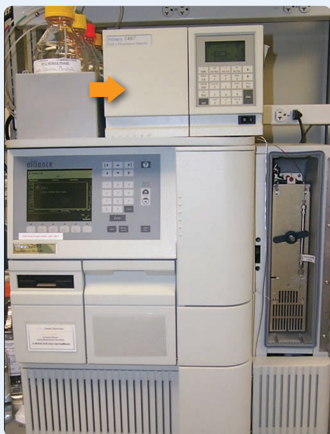
FIGURE 7: Replacing the detector flow cell in a Waters Alliance
