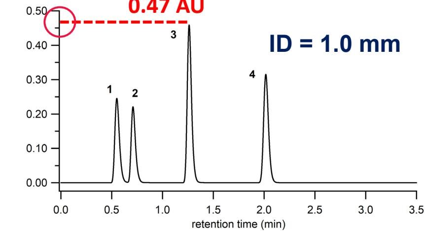
**Signal increases as i.d. decreases with identical sample load on column.**
