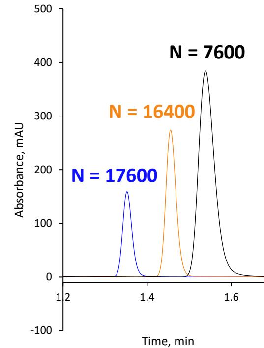
*In move from 2.1 mm i.d. to 1.0 mm i.d., signal increases and viscous friction decreases, but there is a significant loss in efficiency primarily due to extracolumn effects. 1.5 mm i.d. columns can provide a compromise between these effects.*
