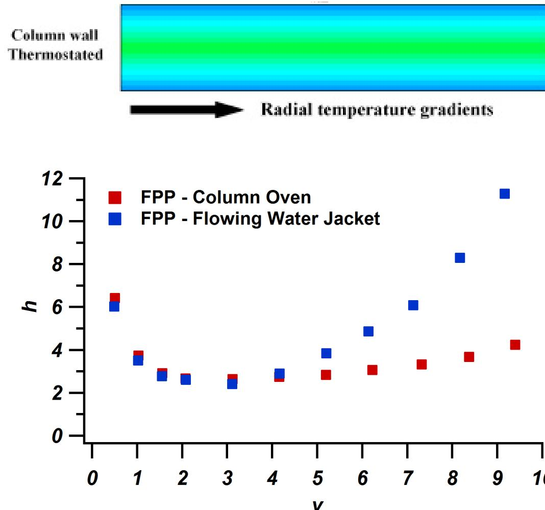
***Radial Thermal Gradients are maximized in (quasi)-isothermal environments:***
