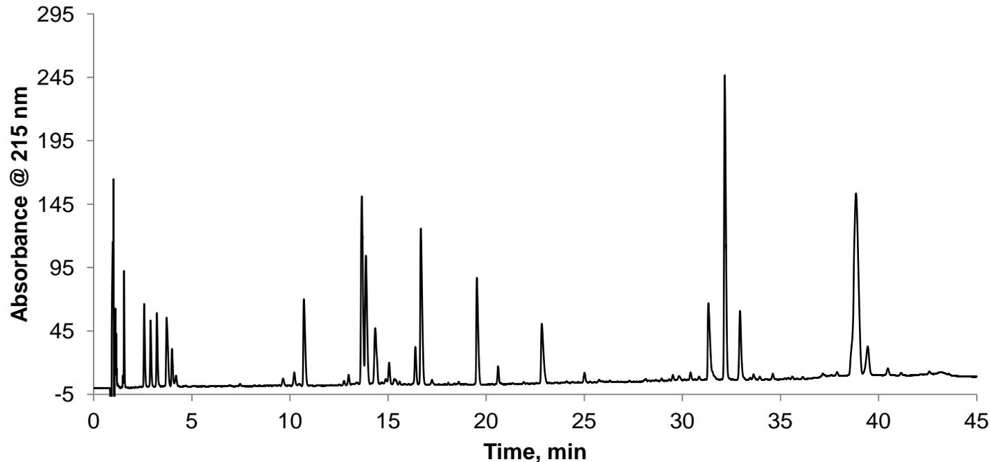
The extremely low back pressure of the HALO-5 Peptide ES-C18 column enables fast, efficient proteomic separations with a low potential for plugging.
