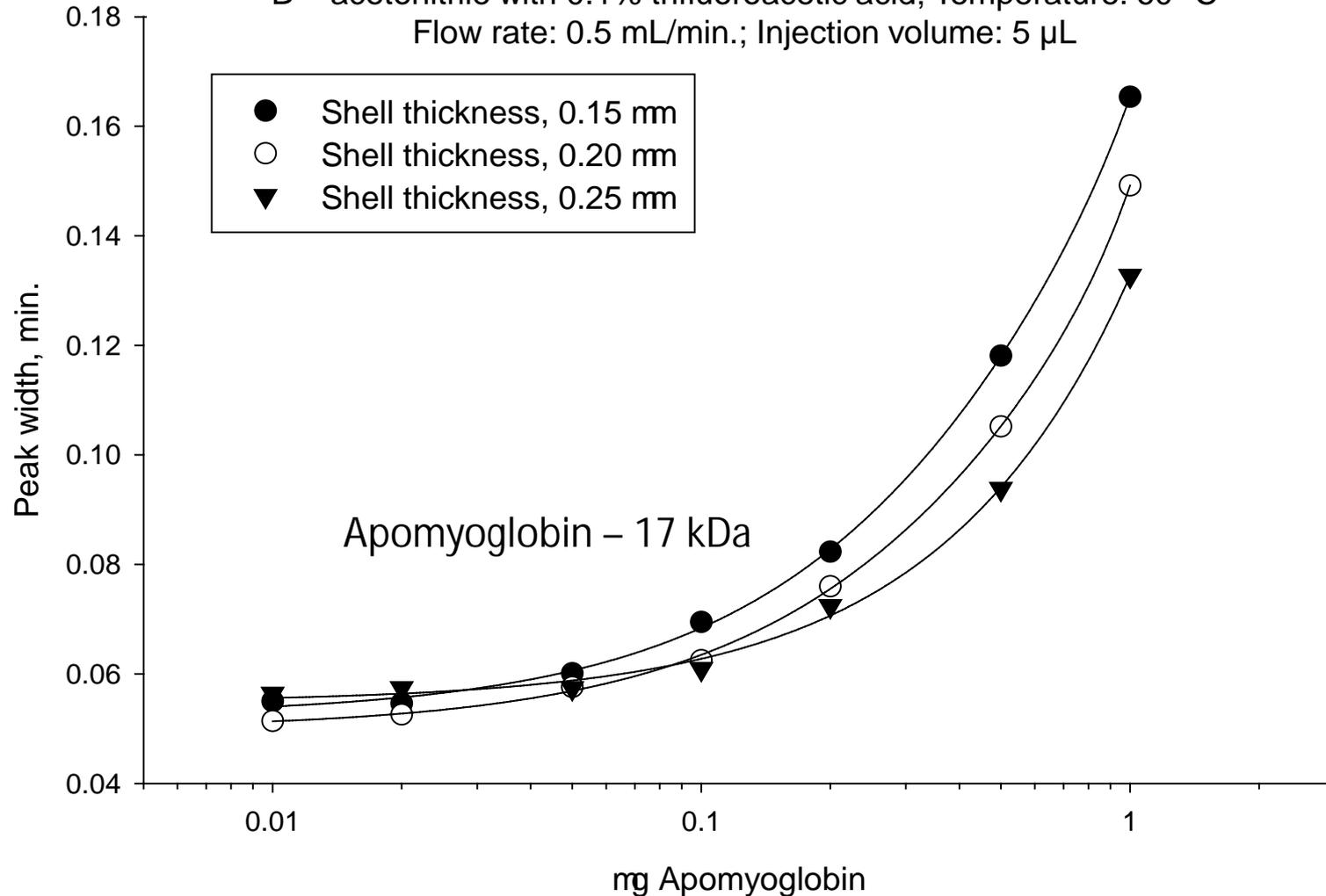
The particle with 0.20  $\mu$ m shell thickness offers a compromise between sample loadability and retention, as well as an optimized diffusion path for large MW biomolecules.
