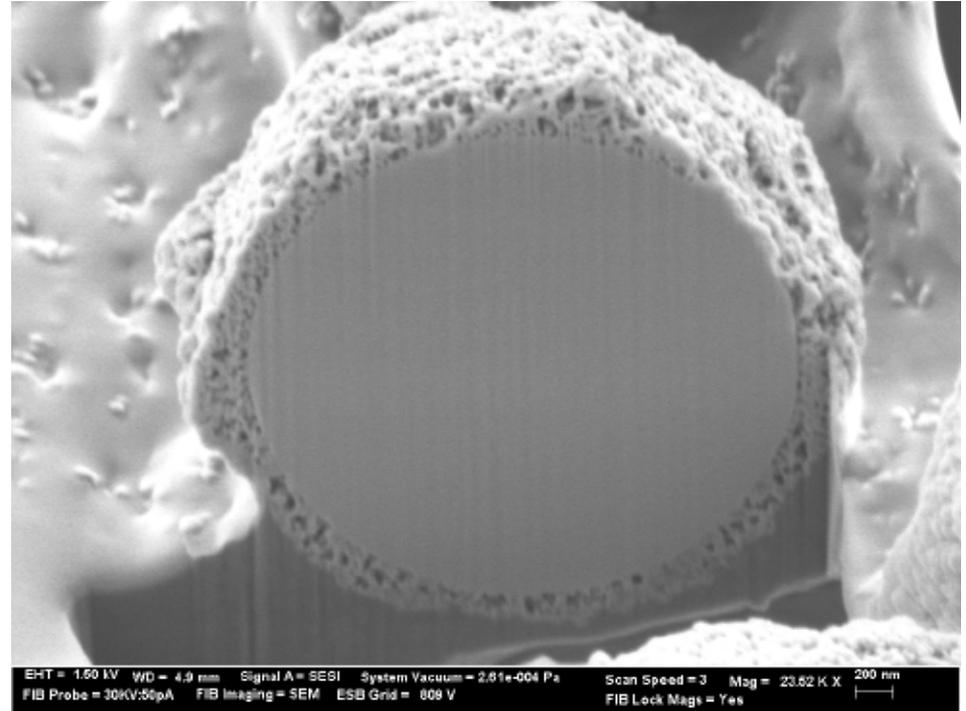
**FIB (Focused Ion Beam) sliced particle**
