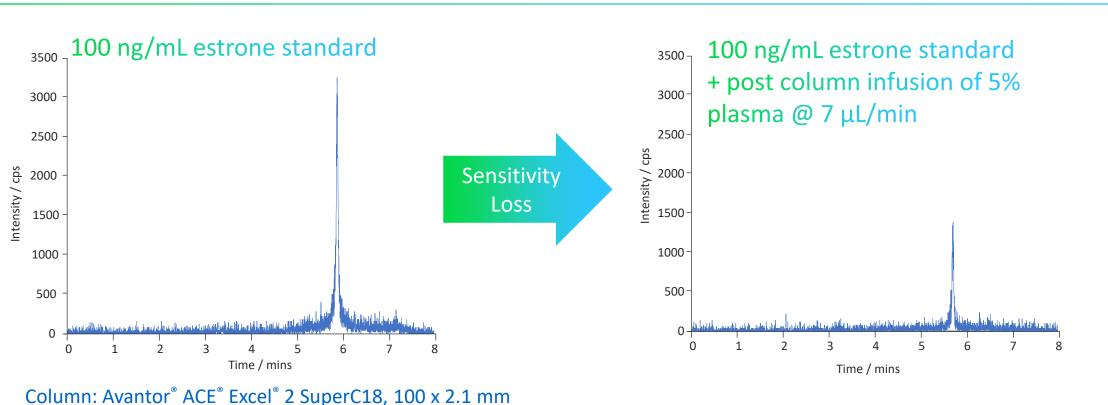
bbile Phase: A: 20 mM NH<sub>4</sub>CH<sub>3</sub>CO<sub>2</sub> (aq) B: 20 mM NH<sub>4</sub>CH<sub>3</sub>CO<sub>2</sub> in MeOH/H<sub>2</sub>O (90:10) radient: 2%B for 1 min, then 2-60%B in 5 mins, Flow Rate: 0.4 mL/min, Injection: 1.0 µL, Temperature: 50 °C
