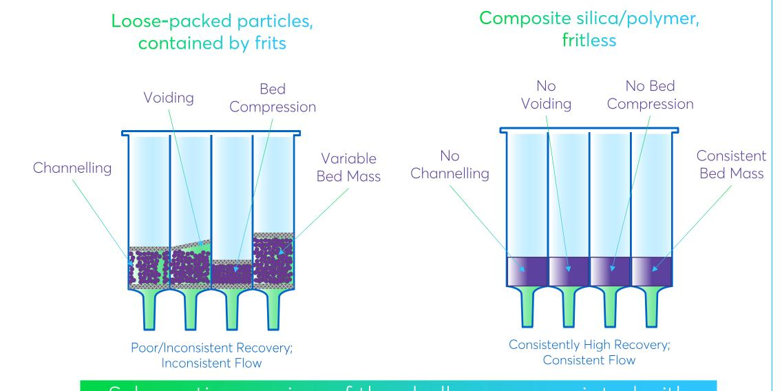
Schematic overview of the challenges associated with loose packed SPE compared to composite SPE
