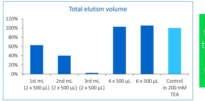
Sequential elution of thymidine 20mer from the WAX SPE cartridge demonstrates that more than one elution step is required
