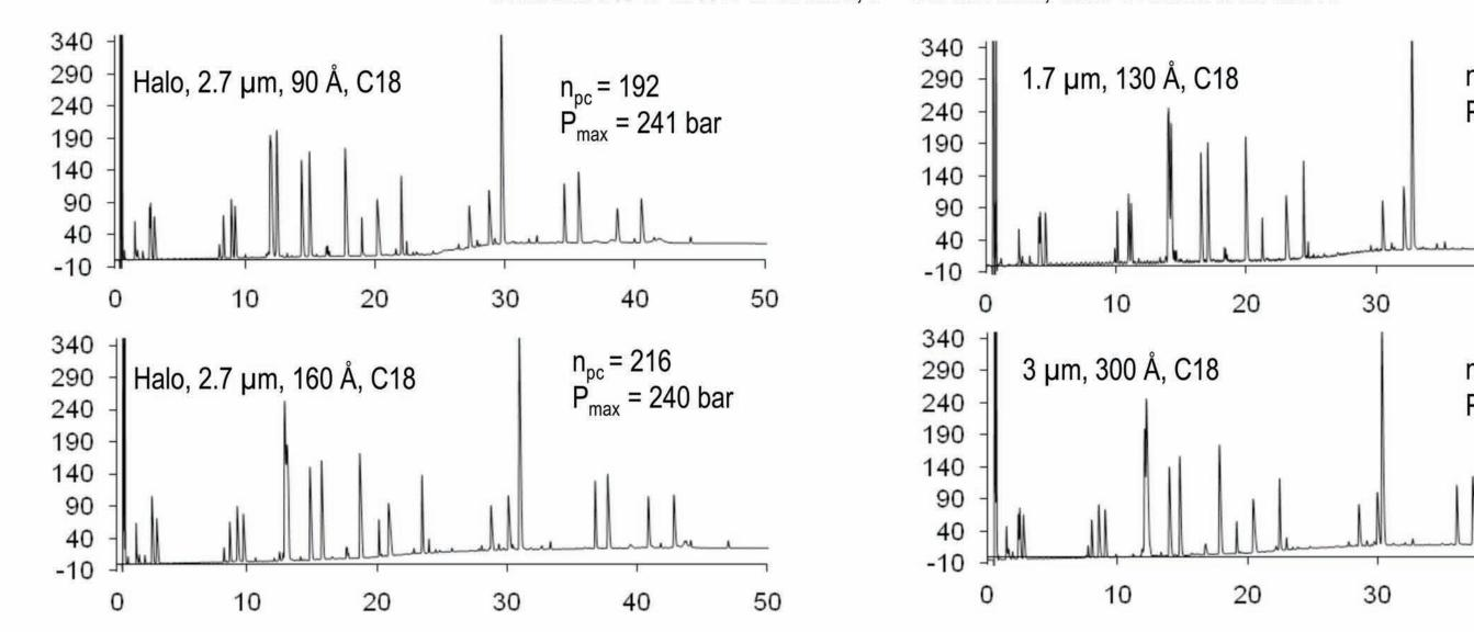
• The peak capacity of HALO Peptide ES-C18 is comparable to that of sub-2-µm, but with less than one half the back pressure. • Compared to a totally porous 3 um column material, HALO Peptide ES-C18 gives better resolution of the small, early eluting tryptic digest fragments, and high flow rate tolerance.
