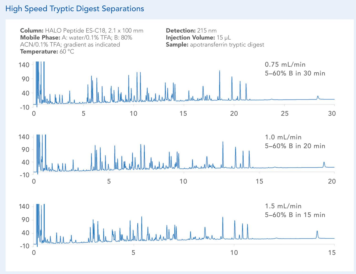
• The short diffusion path of Fused-Core particles allows the use of high mobile phase velocities for fast separations, without sacrificing resolution.
