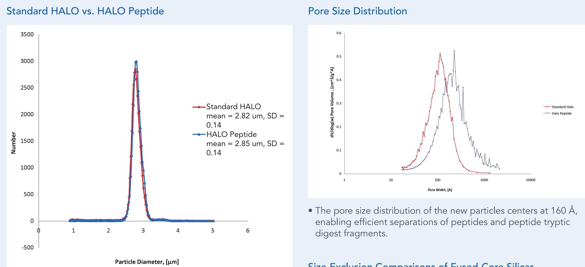
Particle sizes and distribution data were collected on a Multisizer 3 Coulter Counter (Beckman Coulter, Fullerton, CA) using a standard procedure. The results show that the particle size and distribution of HALO Peptide is very similar, if not identical, to Standard HALO. The extremely narrow particle size distribution of both Standard HALO and HALO Peptide have standard deviations that are 5% of the mean.
