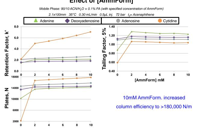
Appropriate AmmForm concentration resulted in highly efficient and symmetrical peaks, along with adjustable selectivity
