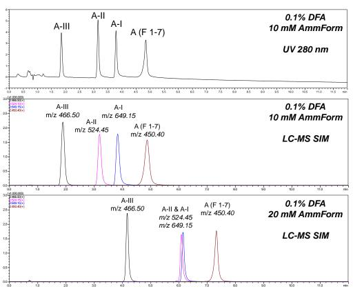
Retention and resolution can be manipulated by choice of DFA or FA, and by adding AmmForm
