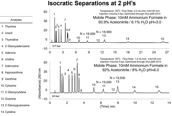
Fully resolved isocratic separation of all 15 components was achieved on a high efficiency Penta-HILIC column, using an appropriate low ionic strength mobile phase modifier
