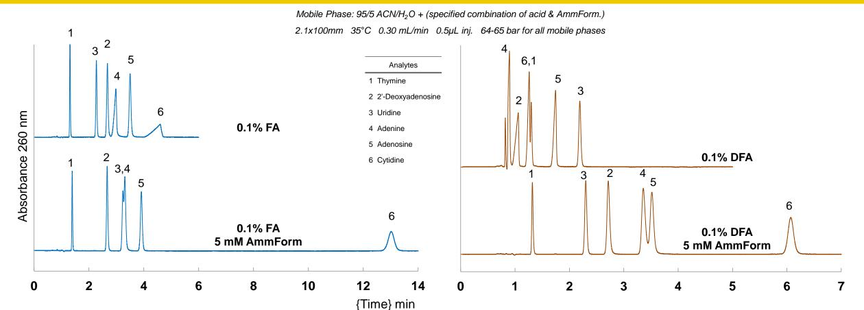
The combination of acidic modifier and AmmForm provides on average higher column efficiency, improved tailing factor, and increased retention. 0.1% DFA and 5mM AmmForm demonstrated the best separation under these conditions.
