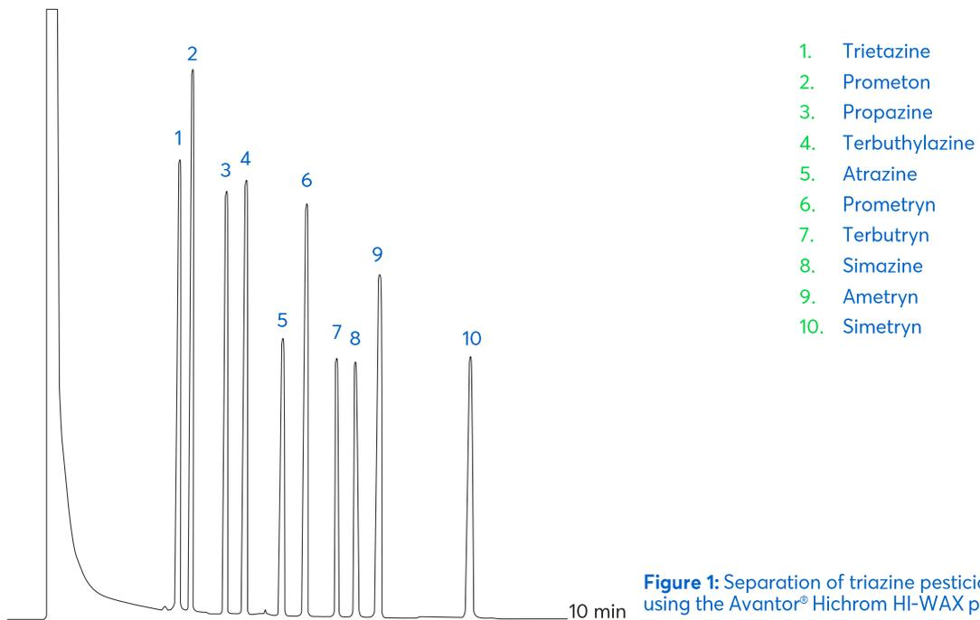
**Figure 1:** Separation of triazine pesticides using the Avantor<sup>®</sup> Hichrom HI-WAX phase.
