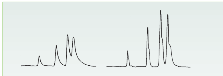
FIGURE 3. Peak distortion of all peaks in the chromatogram due to a partially blocked frit or column void.
